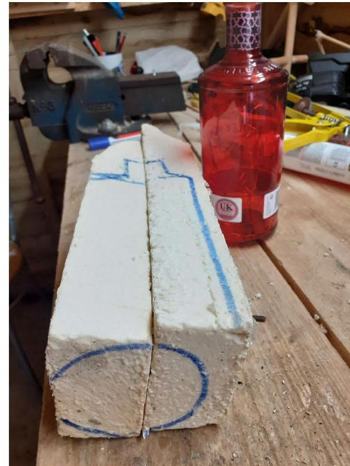
Stage A): Stick foam together with double-sided tape and draw
