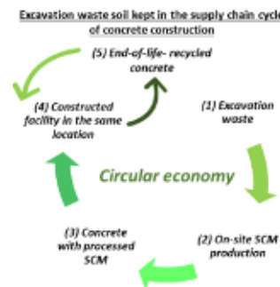
(b) Circular use of Excavation waste
