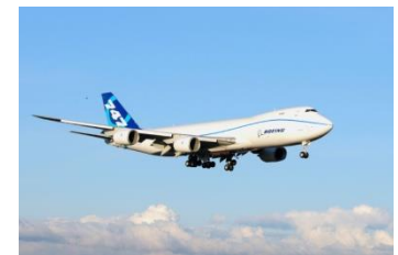
Aluminium alloys are used to make aircraft frames and body panels. ( http://commons.wikimedia.org/wiki/File:Boeing_747-8_N747EX_First_Flight_2-8-2010.jpg )
