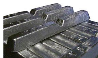
Cast aluminium ingots for further processing. ( https://commons.wikimedia.org/wiki/File:Aluminium_bar.jpg )
