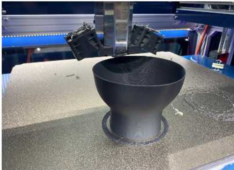
High Flow 3D Printed Socket Liner, NinjaTek Chinchilla
